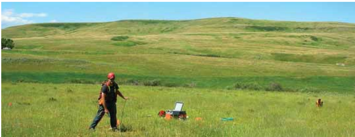
Figure 7. Testing true amplitude seismic response in the field to calibrate monitoring instruments
